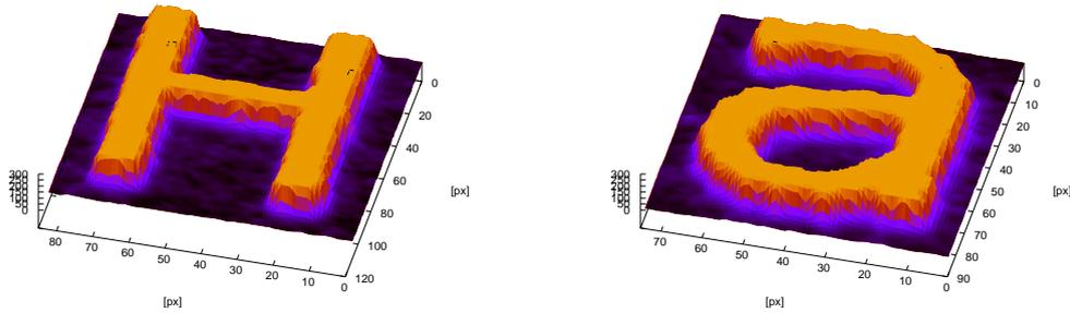
Figure 3.4: Exemplary surface plots of the inkjet printed characters "H" and "a" scanned with a resolution of  $800dpi$ . A light blurring and an increased roughness at the character edges is observable.
