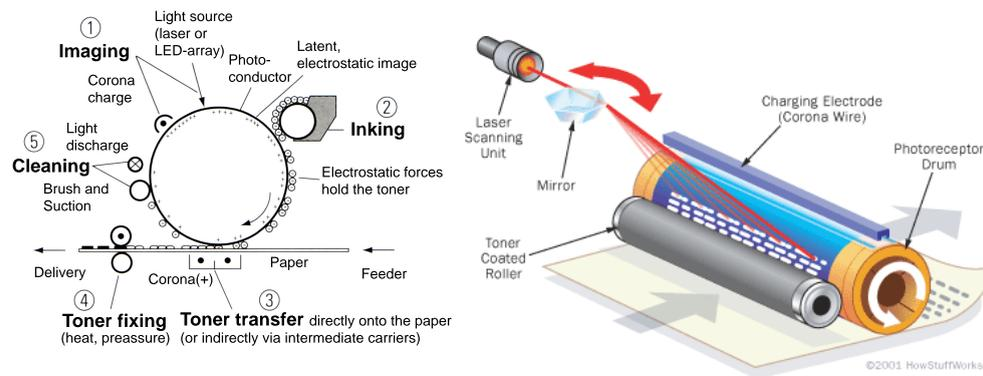
Figure 3.3: The electrophotographic printing process: (l) basic elements of electrophotographic printing as illustrated by Kipphan [40] (r) charging of the photoconductor drum.
