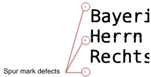
Figure 3.9: Typical printer traces left at a document image that are caused by the physical properties of the printer. The image above shows exemplary spur marks induced by the gears of the printing device.
