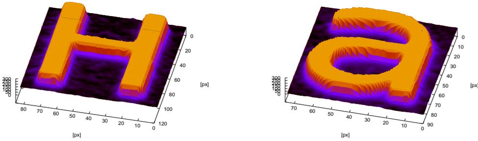
Figure 3.6: Exemplary surface plots of the electrophotographic printed characters "H" and "a" scanned with a resolution of  $800dpi$ . A sharp transition between character and non-character regions is observable.
