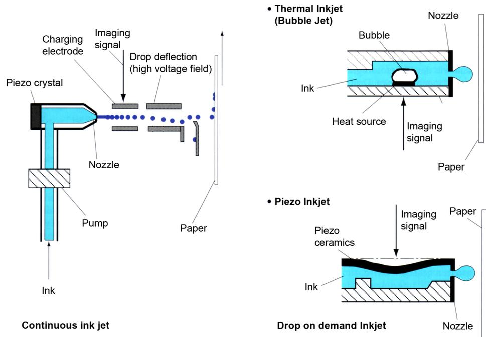
Figure 3.2: The inkjet printing process: (l) basic elements of continuous inkjet printing and (r) basic elements of drop on demand inkjet printing as illustrated by Kipphan [40].
