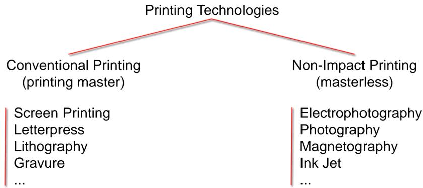
Figure 3.1: Taxonomy of different printing technologies according to Kipphan [40]. A distinction is made between technologies that touches the printing substrate to create an image (Conventional printing) and those that do not (Non-impact printing).
